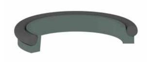
K706 is a two piece acting wiper which consists of one special designed thermoplastic ring and an o-ring as energizing element. K706 ensures that foreign particles do not penetrate into the hydraulic systems, avoiding wear and damage to all internal components including seals.
