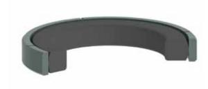
K755 is a two piecedouble acting piston seal which consists of one energizing elastomer ring and special mixture thermoplastic ring.
