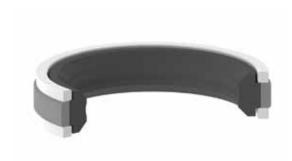
K48 is a four piece double acting heavy duty piston seal which consists of one TPE profile ring, one elastomeric nitrile rubber to pre load sealing element and two thermoplastic back-up rings.
