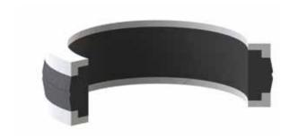
K505 is a three piece double acting compact seal which consists of one fabric reinforced elastomeric sealing element and two thermoplastic guide back-up rings.
