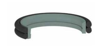
K705 is a three piece single acting wiper which consists of one special mixture PTFE profile ring and two o-rings as energizers. K705 ensures that foreign particles are not introduced into the hydraulic systems, avoiding wear and damage to all the internal components including seals.
