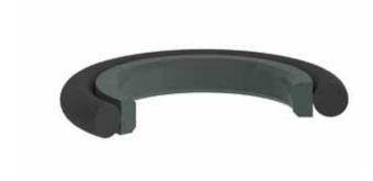
K709 is a two piece double acting rod seal which consists of one special mixture PTFE profile ring and an o-ring as an energizing element.
