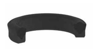
K39 is a single acting rod seal which consists of reinforced cotton fabric and nitrile rubber vulcanized together forming an integral sealing element.
